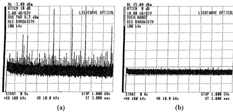
CThO47 Fig. 2. Longitudinal-mode frequencies of the ring resonator measured by a passive homodyne method without (a) and with (b) MRC.
