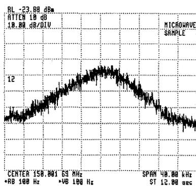
**CThO48 Fig. 3.** Measured linewidth of the FBG ring lasers by using a self-heterodyne method.
