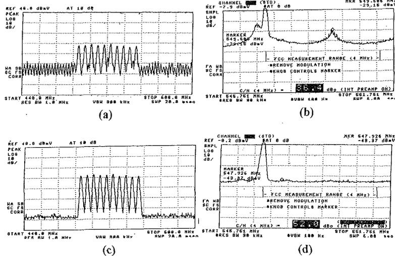
CThO47 Fig. 3. The received rf-output spectra for a 10 NTSC system transmission of full span (a), and the 78th channel at 547.25 MHz (b) with the transmitter without MRC technique and of full span (c), and the 78th channel at 547.25 MHz (d) with the transmitter using MRC operation.
