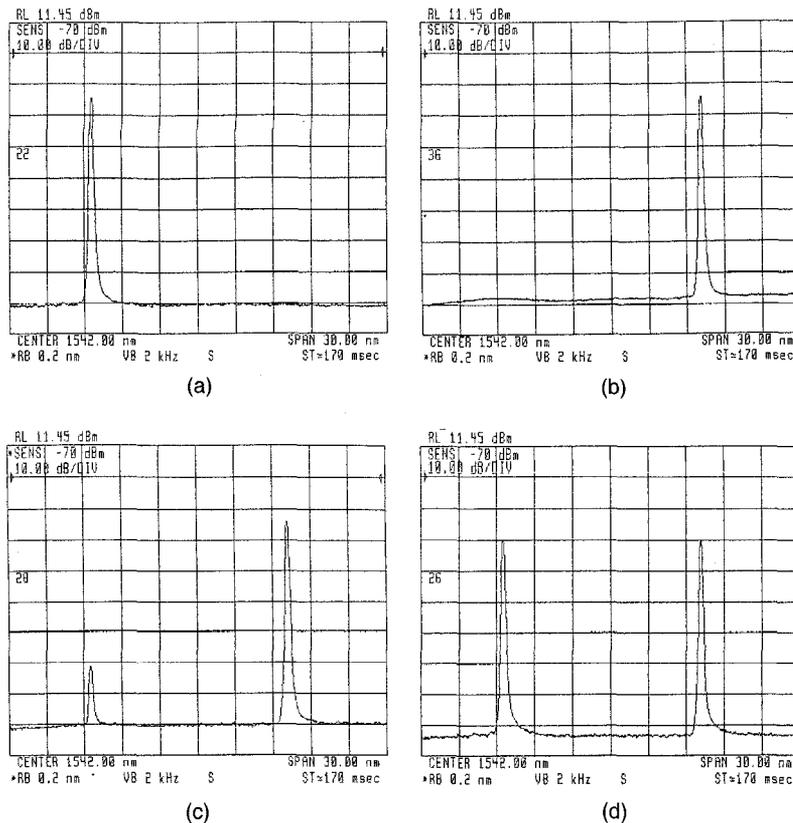
**CThO48 Fig. 2.** Output spectra of the dynamically wavelength-switching FBG ring lasers. OSW switched to port 1 (a), port 2 (b), or port 3 [(c), (d)], but a microbender for gain-equal control has been inserted in (d).
