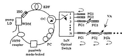
CThO48 Fig. 1. Experimental setup of the proposed gain-equal multiwavelength ring lasers. EDF: erbium-doped fiber. FG: fiber grating. ISO: optical isolator. OC: optical circulator. PC: polarization controller. VA: microbender as variable attenuator.
